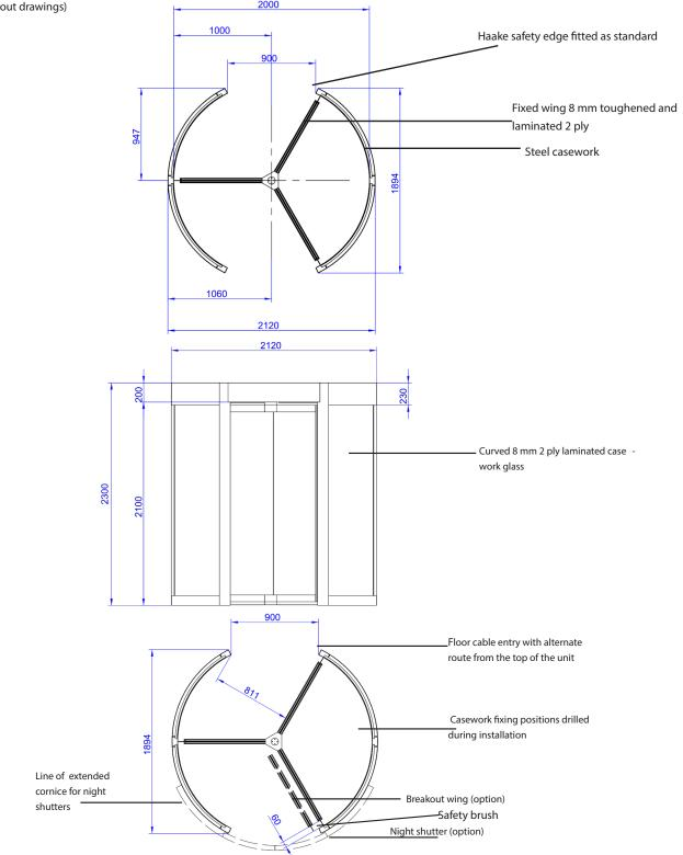
Product is delivered in a kit form and requires lifting equipment. Approx. Weight 710 kg (for installation details, please refer to installation layout drawings)
