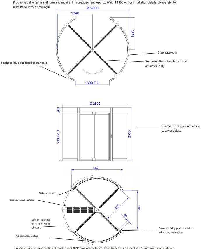
Concrete Base to specification at least (cube) 30N/mm2 of resistance. Base to be flat and level to +/-5mm over footprint area. Dimensions to be > 2900 x 2900 x 150 deep min. (units in mm).
