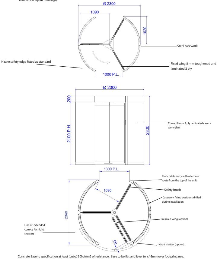
Dimensions to be >2400 x 2400 x 150 deep min. (units in mm).
