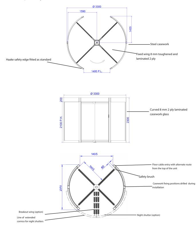
Concrete Base to specification at least (cube) 30N/mm2 of resistance. Base to be flat and level to +/-5mm over footprint area. Dimensions to be >  $3400 \times 3400 \times 150$  deep min. (units in mm).
