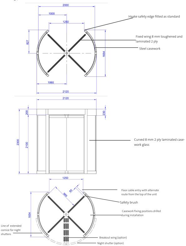
Concrete Base to specification at least (cube) 30N/mm2 of resistance. Base to be flat and level to +/-5mm over footprint area. Dimensions to be > 2250 x 2250 x 150 deep min. (units in mm).
