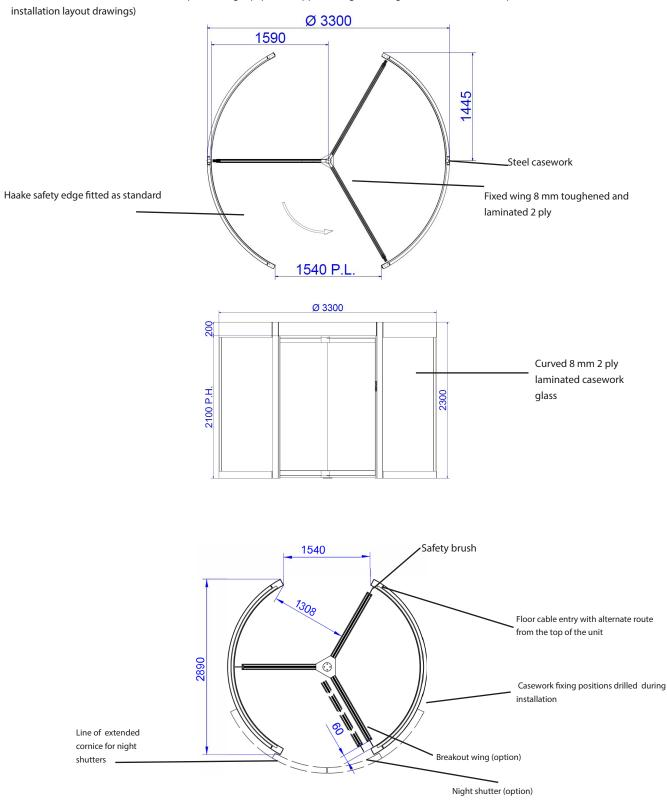
Product is delivered in a kit form and requires lifting equipment. Approx. Weight 1300 kg (for installation details, please refer to
